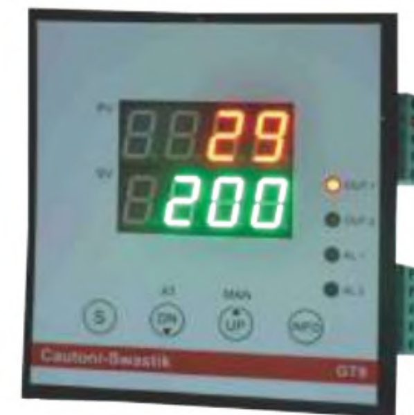
TEMP. CONTROLLER CARD
