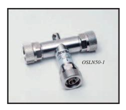
The OSL series open/short/load are used on the test port of the Site Master Series of handheld instruments to establish a reference for accurate measurement. When used with a Site Master, the open/short and load reflection over a swept frequency range can be automatically averaged to enhance measurement accuracy. OSL series Open/short/load comes in both N(Male) and N (Female) connector configuration and consist open on one end, short on other and Load on the tee section.
