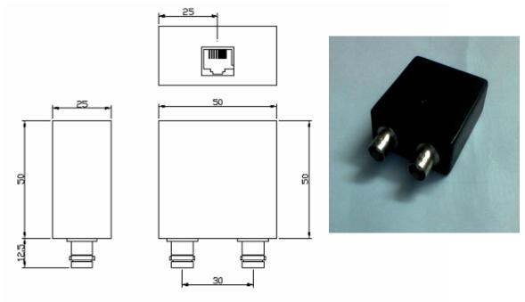
RJ45 Connectors Contacts:: Phosphor Brouce plated Ni/Au
