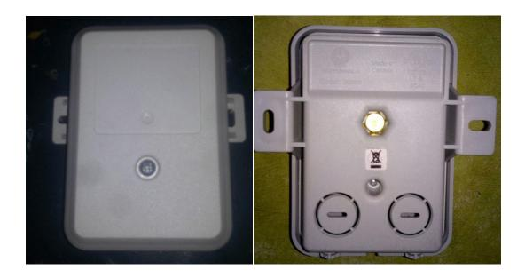
The Canopy Surge Suppressor can be used in conjunction with all Canopy products (AP, SM and BH). A surge suppressor is a device inserted in the alternating current (AC) utility line and/or telephone line to prevent damage to electronic equipment from voltage "spikes" called transients. A more accurate term for this type of device is "transient suppressor."
