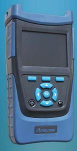
SAT-18C1 palm OTDR is the newest instrument designed for testing FTTx network. It's mainly used to measure the physical characteristics of optical fiber under test, such as the length, the transmission loss and the splice loss etc.. It can also locate the faults or breaks of optical fiber. It's widely applied in the manufacture, construction and maintenance in optical fiber communication system.
